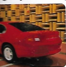
Hemi-anechoic chambers are used to evaluate vehicle noise through reflected sounds.
